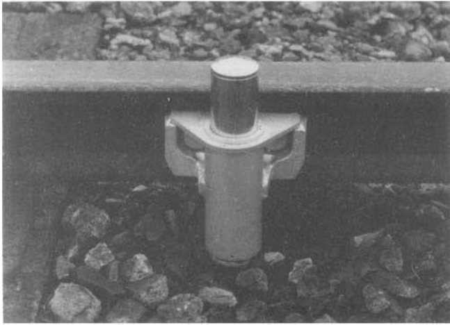
Fig. 6 The prototype capsule retarder
