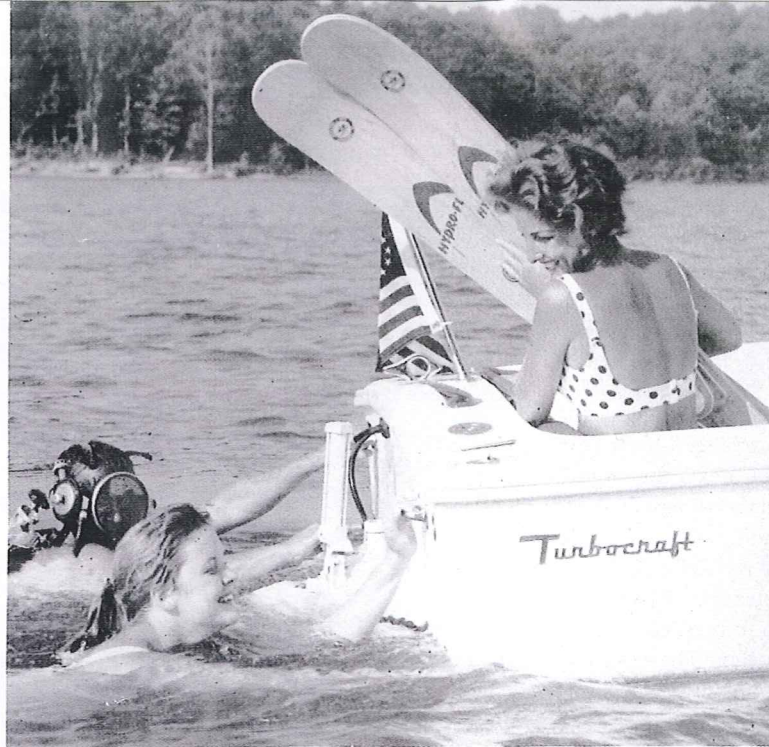
Far left: What shear pin? The waterjet unit, with no propeller, meant incredibly low draught, resulting in stunts like this Left: No propeller also meant no danger to swimmers, so it was an ideal boat for waterskiing
