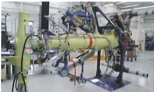
The next main gear ready for delivery to DGA, Toulouse for Drop Testing and subsequently installed in the DGA Drop Test rig.
