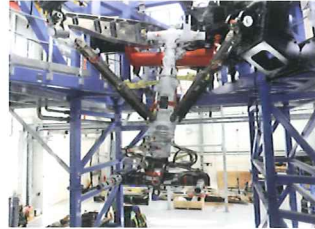
The first gear set delivered to Airbus for the Systems Test Rig and subsequently installed in the rig.
