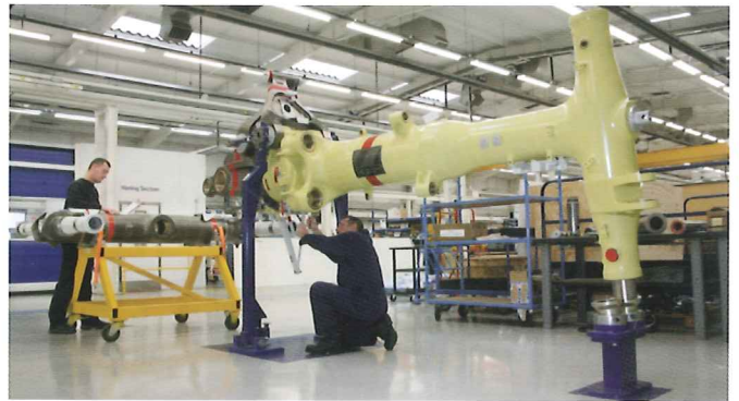
The recently modified test rig at Gloucester for the A350 Fatigue Test and the final preparations to the gear before it is installed in the rig.
