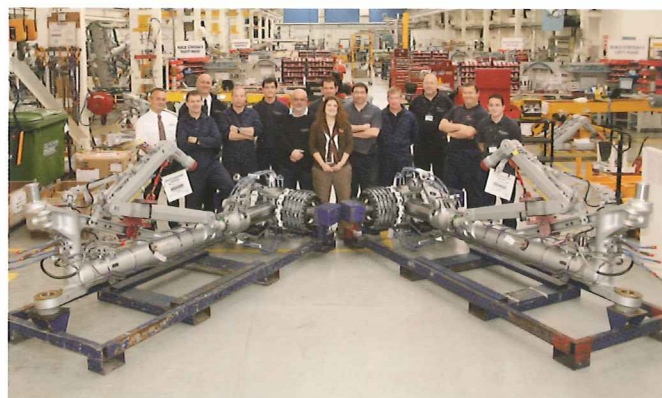
1st Mexican A320 main fittings assembled on main gear
