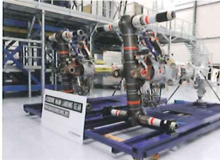
The first gear set delivered to Airbus for the Systems Test Rig and subsequently installed in the rig.
