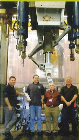
Completion of A340-500/600 High Gross Weight Centre Landing Gear fatigue test.
