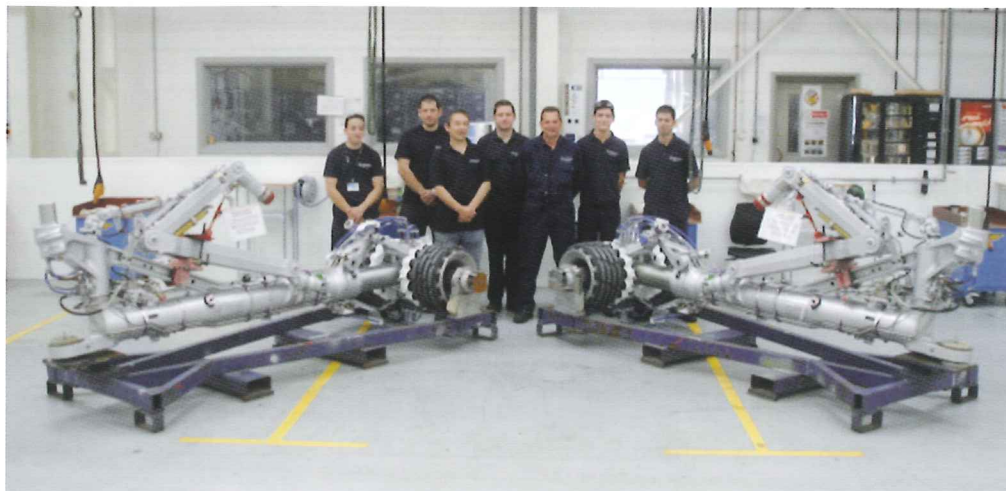
1st Mexican A321 main fittings assembled on main gear
