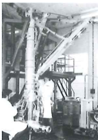
A320 main gear with side stay and lock links fitted
