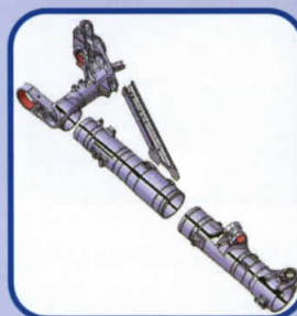
Figure 7: Main fitting Concept showing potential Welded Joint Locations (Design property of Messier-Dowty)
