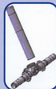
Figure 8: Sliding Member Concept showing potential Welded Joint Locations (Design property of Messier-Dowty)
