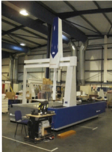
The picture above shows the first CMM in readiness for the preliminary tests to verify accuracy before being despatched.
