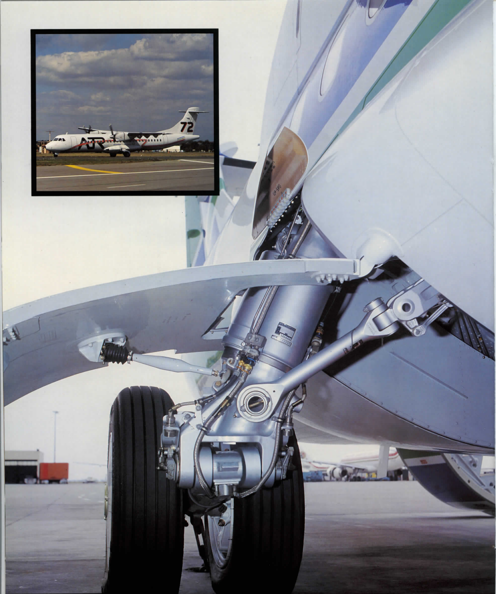
Messier makes the main landing gear for the ATR 72 regional turboprop aircraft at Bidos, France.
