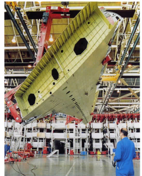
Pictured is an A340 wingbox being moved out of assembly jig at the Airbus manufacturing facility at Chester
