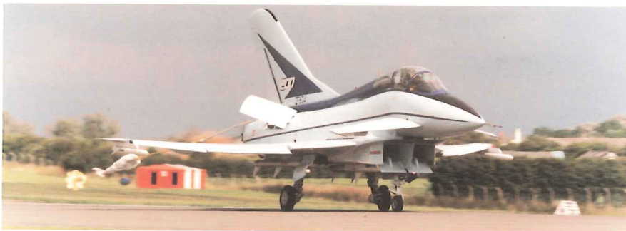
British Aerospace EAP main and nose landing gears. The EAP was the development aircraft and forerunner to the Eurofighter.
