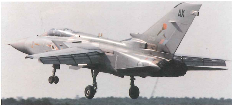
Panavia Tornado main and nose landing gears.
