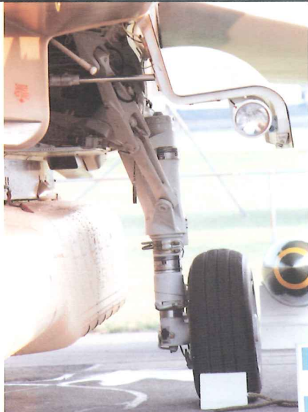
Panavia Tornado main and nose landing gears.
