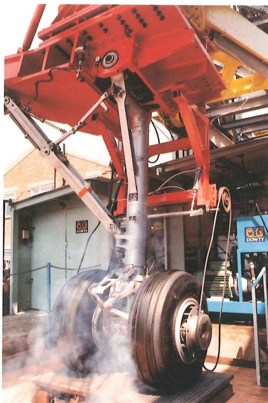
Drop testing the A320 main landing gear in Europe.
