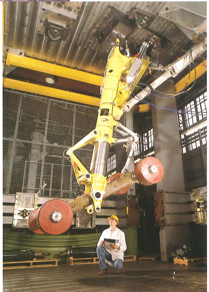
Retraction testing of A340 main landing gear in Europe.
