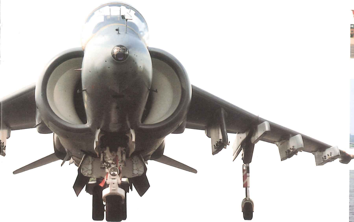
British Aerospace Harrier II and McDonnell Douglas AV-8B main, nose and wing gears.
