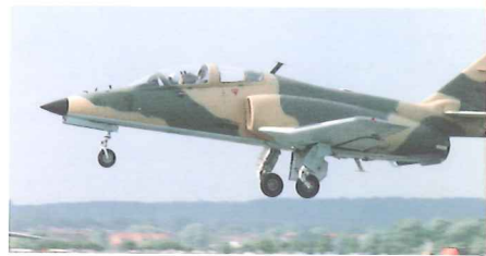
Casa C-101 main and nose landing gears.
