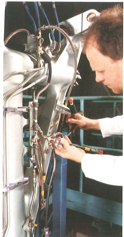
Fitting landing gear harness.
