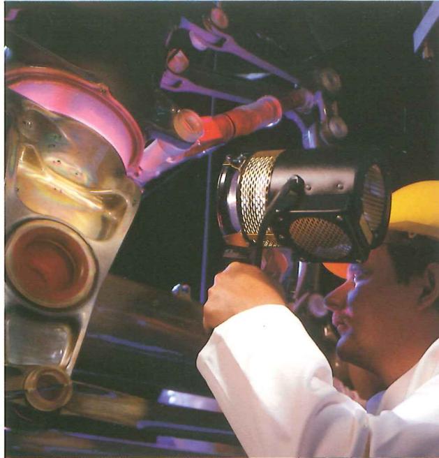
Photo-elastic testing, used by Dowty to verify stress analysis programs during the development of a landing gear.
