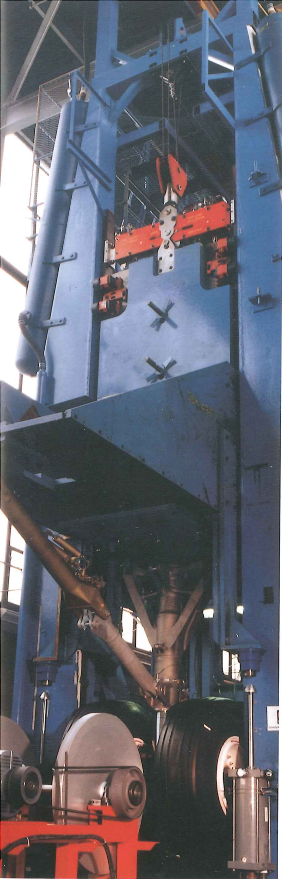
Drop testing the A340 centreline landing gear in North America.
