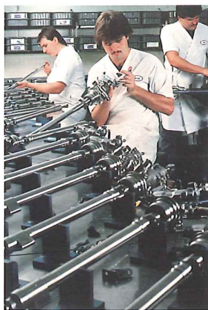
Assembly of Boeing 737-300 thrust reverser actuators.
