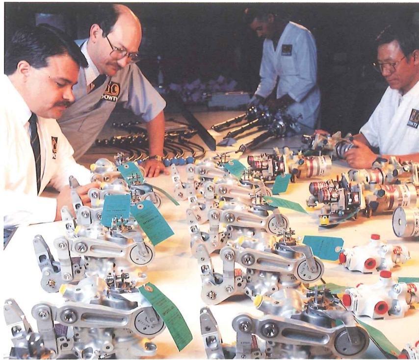
Detailed final assembly and inspection of actuators.
