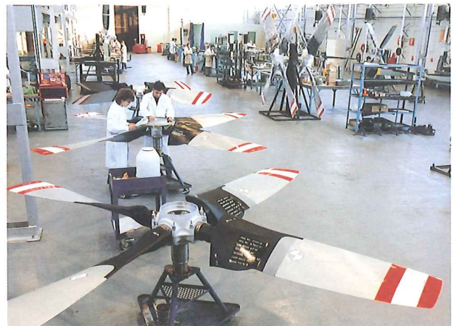
C130 propellers undergo repair and overhaul.
