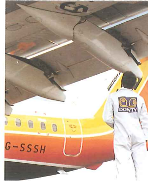
Dowty's high lift system for the British Aerospace 146 trailing edge flaps, signalled and monitored by digital electronics.
