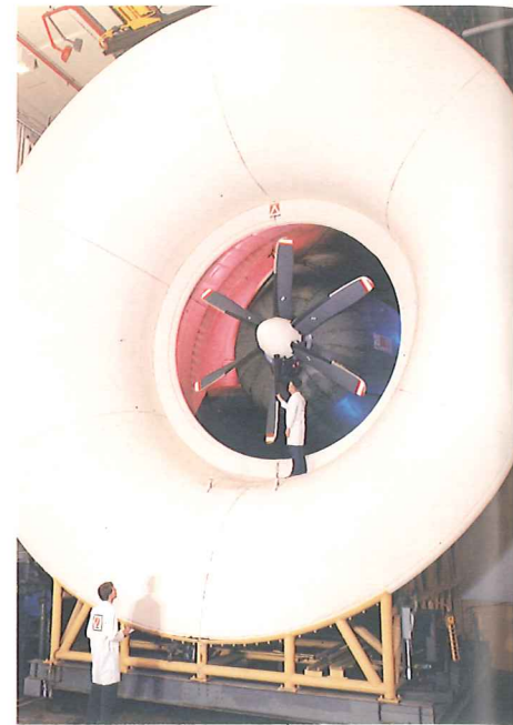
Testing a large composite propeller in an Allison engine test cell.
