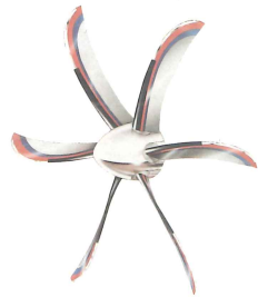
Dowty composite propeller for Saab 2000
