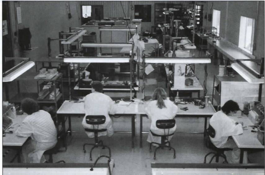
A cell concept. Again with work benches side by side in a "U" shape line, continuous flow is inevitable. The cell cultivates a focus on team work, feedback and sharing of ideas. These are currently used in the mechanical assembly areas where subassembly integration is performed.
