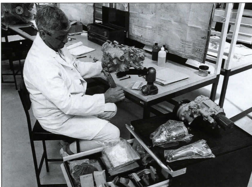
Single level assembly of the RB199 Reheat Control Unit using a fastener pack. Each item is individually bagged and labelled in the correct assembly sequence.
