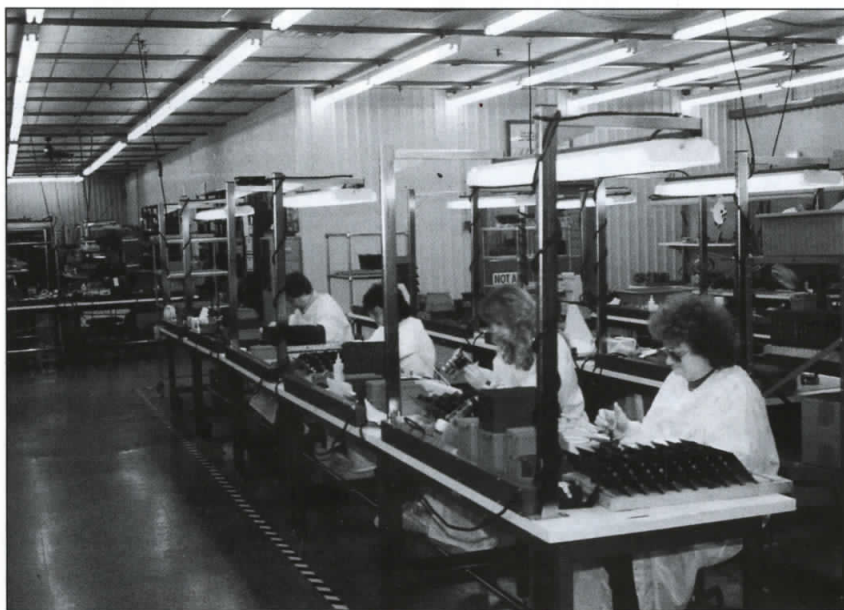
A progressive assembly line in the P.C.B. assembly area. Note: The work benches are along side one another. This produces a continuous flow of work-in-process (W.I.P.).
