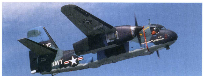
The Grumman S-2 Tracker undergoing flight trials with Dowty Rotol composite bladed propellers.
