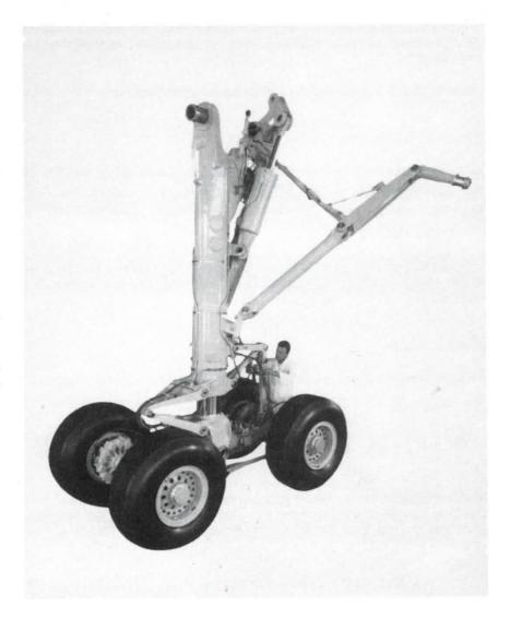
Airbus A330/340 main landing gear mock-up
