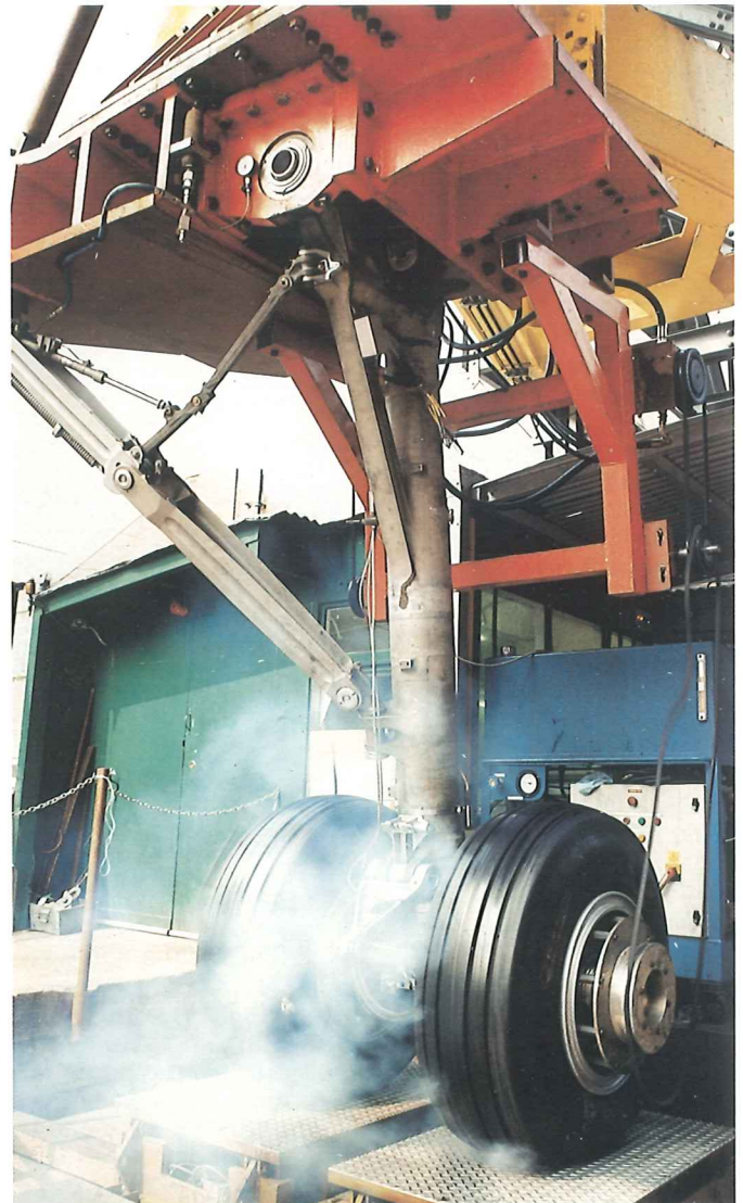
A320 main landing gear on drop test rig
