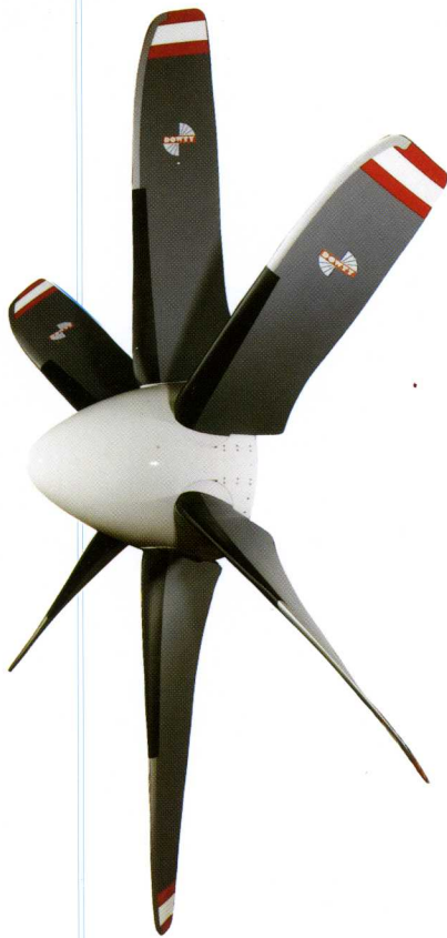
Composite propeller for the Allison T406 turboprop propulsion system
