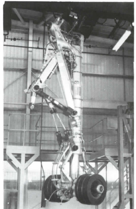
Landing gear set 22 for the A320 aircraft, the first of the 72 tonne landing gear shown as it is lifted from its assembly frame.
