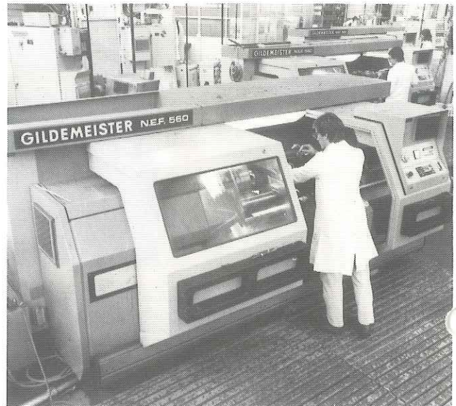
New Gildemeister turning machines in No. 1 Machine Shop
