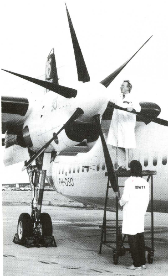
Service engineers checking propeller on Fokker 50
