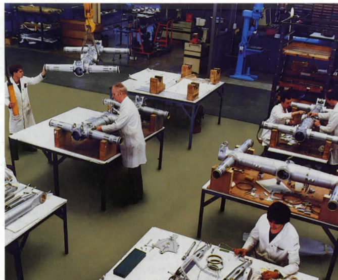
Assembling A310 bogie beam units
