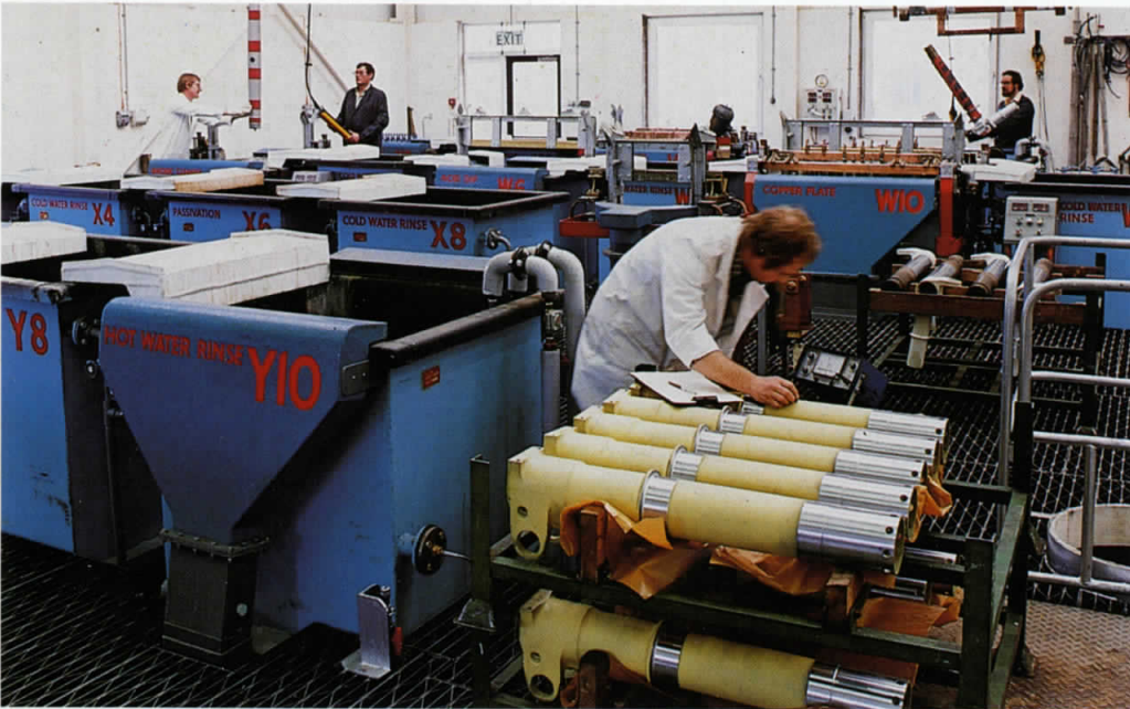
Heat treatment of landing gear reaction bar units
