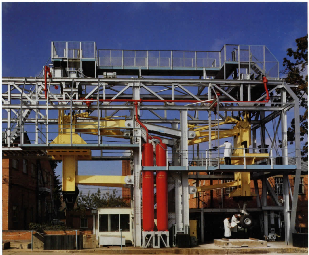
Drop testing rig for landing gear up to 400 000 lb AUW
