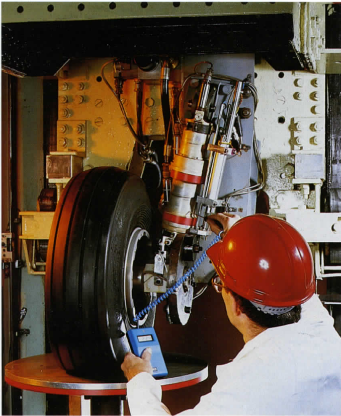
Suspension development testing of model landing gear
