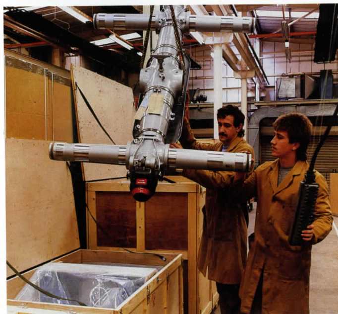
Despatch of A310 main landing gear bogie beam
