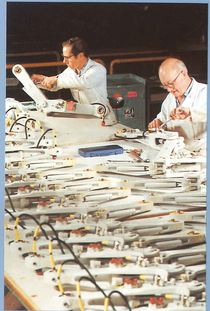
Assembling landing gear lock struts
