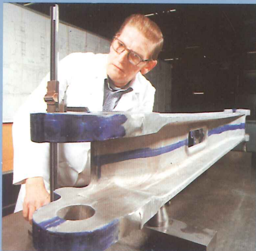
Marking out A310 landing gear upper stay
