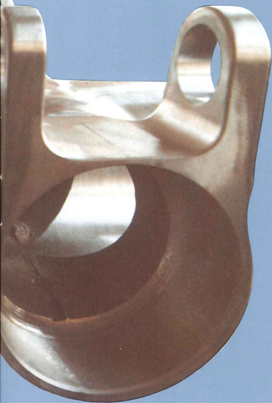
Marking out A310 landing gear upper stay
