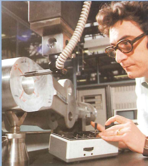
3D inspection of Fokker F.28 main leg
