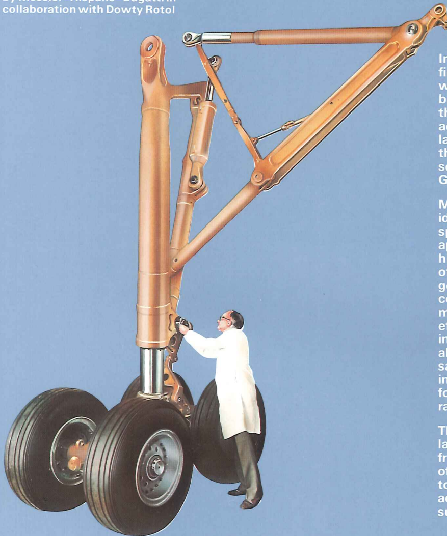
Airbus A310 and below, the main landing gear by Messier-Hispano-Bugatti in collaboration with Dowty Rotol
