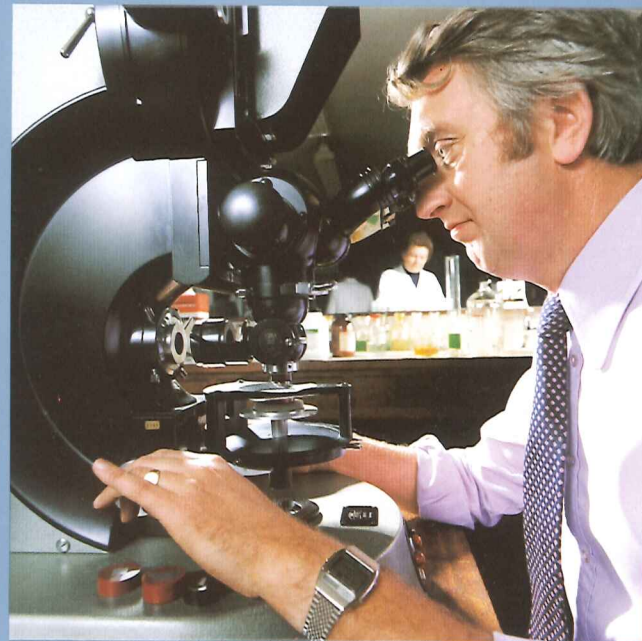
Metallographic examination of landing gear sample
