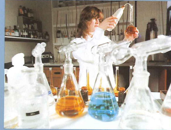
Analysis of chrome plating solution for landing gear
