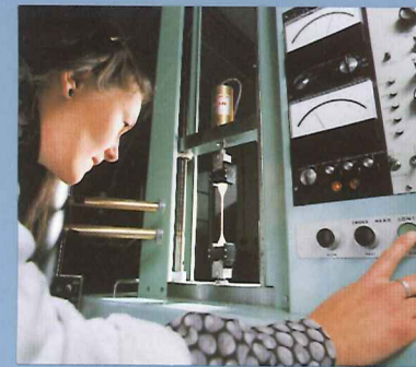
Tensile testing plastics
